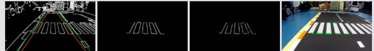
a) Canny Edge Detection + ROI b) Region of Interest c) Hough Line Detection d) Crosswalk detection
