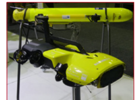
Vision-empowered marine robots COTSbot and RangerBot
