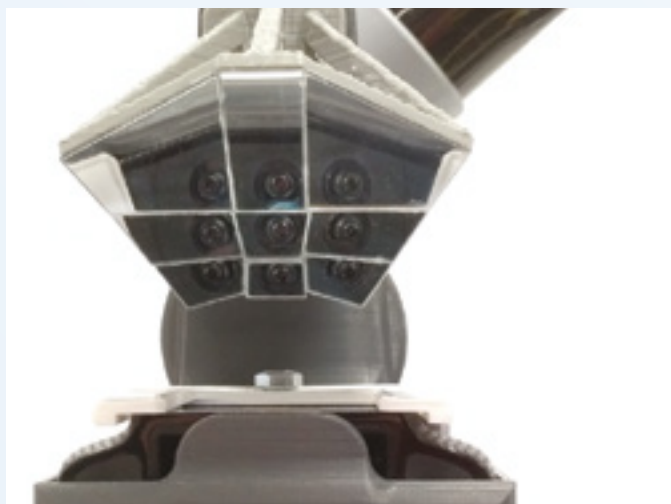
▲ MirrorCam mounted on the Kinova MICO robot manipulator. Nine mirrors in a 3D printed frame to create nine virtual cameras, which provides low-cost video frame-rate light fields.
