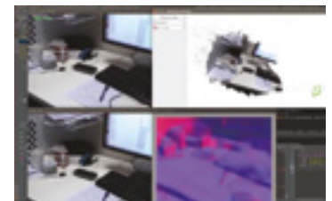
▲ Dense scene reconstruction using CNN-based priors. The camera video feed (left) is processed by a CNN to produce a surface normal prediction (bottom right) and this is fused with geometric information from the image stream to produce a dense reconstruction (top right).
