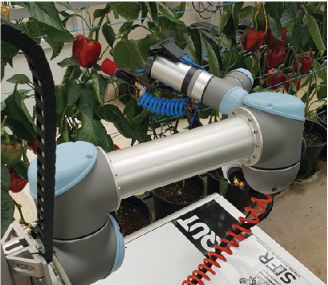
Harvey, a prototype robotic platform for harvesting capsicums, being tested in a protected cropping facility. Harvey was developed as part of a three-year Strategic Investment in Farm Robotics (SIFR) funded by the Queensland Department of Agriculture and Fisheries (DAF).
