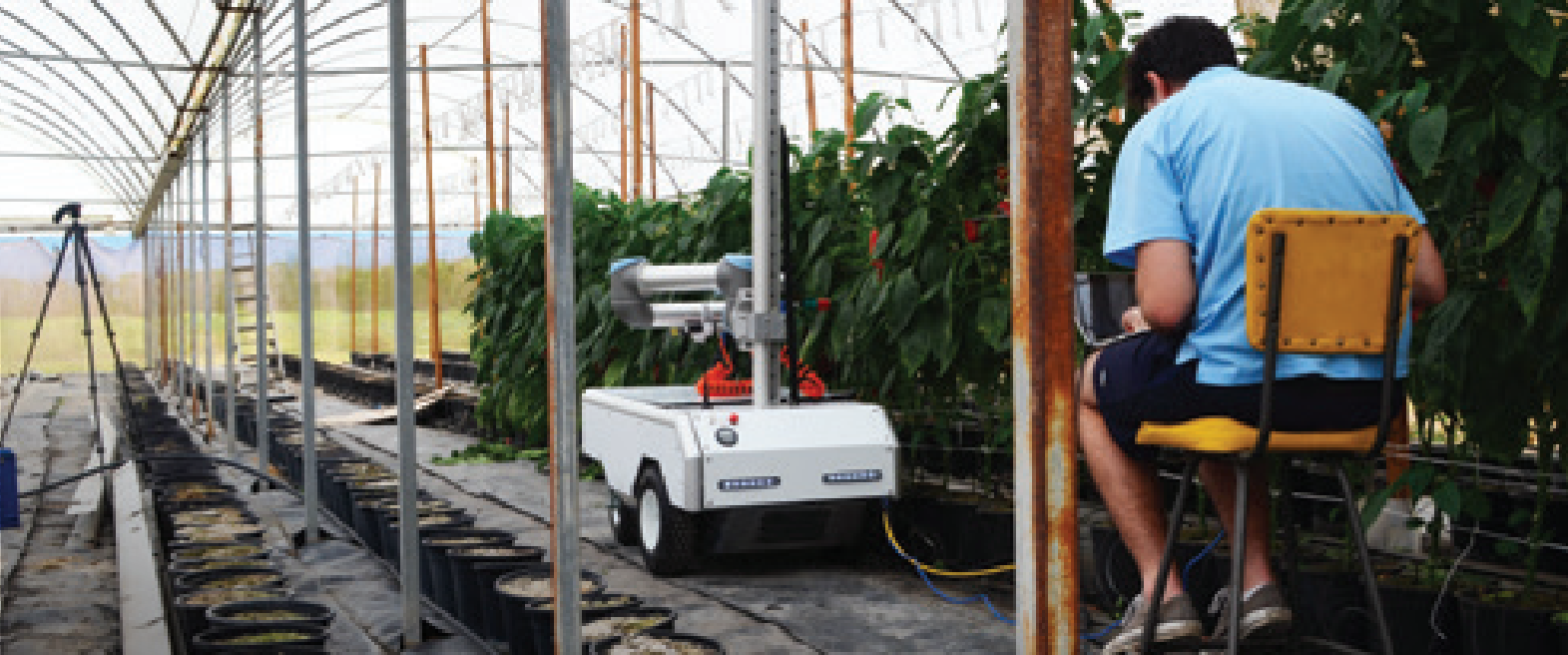
Harvey, a prototype robotic platform for harvesting capsicums, being tested at a Queensland Government protected cropping facility by Chris Lehnert
