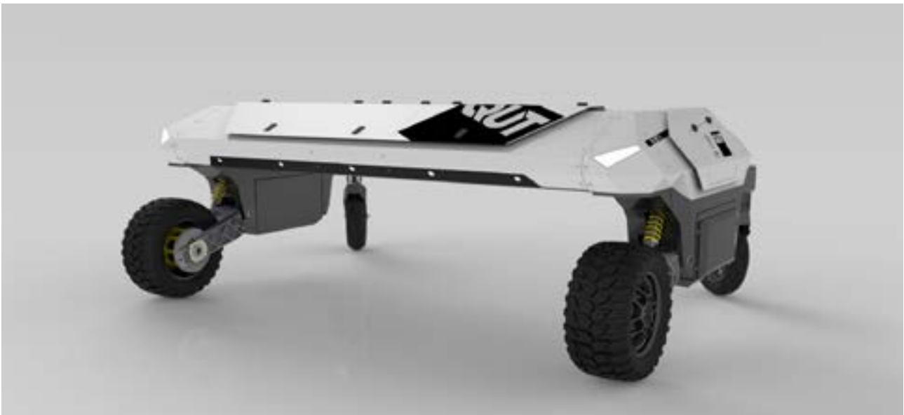
Concept drawing of the prototype broadacre agricultural robot, AgBot II, developed by researchers associated with the ACRV
