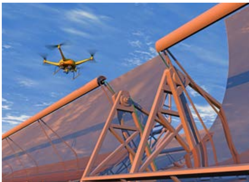
Unmanned Aerial Vehicles (drones) are used to inspect infrastructure assets and identify maintenance requirements
